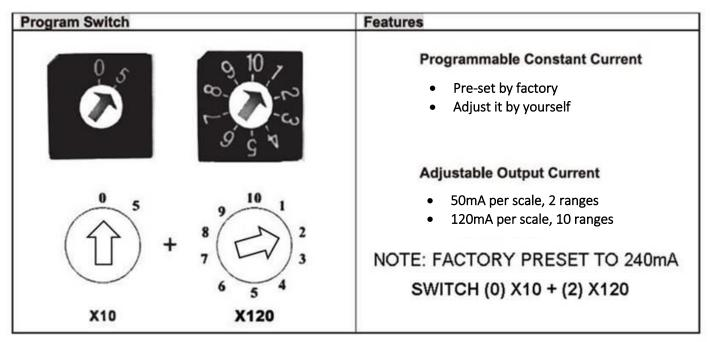
NOTE: LUMENS WILL INCREASE OR DECREASE DEPENDING ON THE PROGRAM SWITCH SETTING. MODIFYING OUTPUT CURRENT WILL INADVERTENTLY CHANGE BATTERY DISCHARGE RATE DURING POWER OUTAGES.
